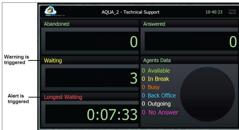
Warning and Alert Triggered on ECS Wallboard
